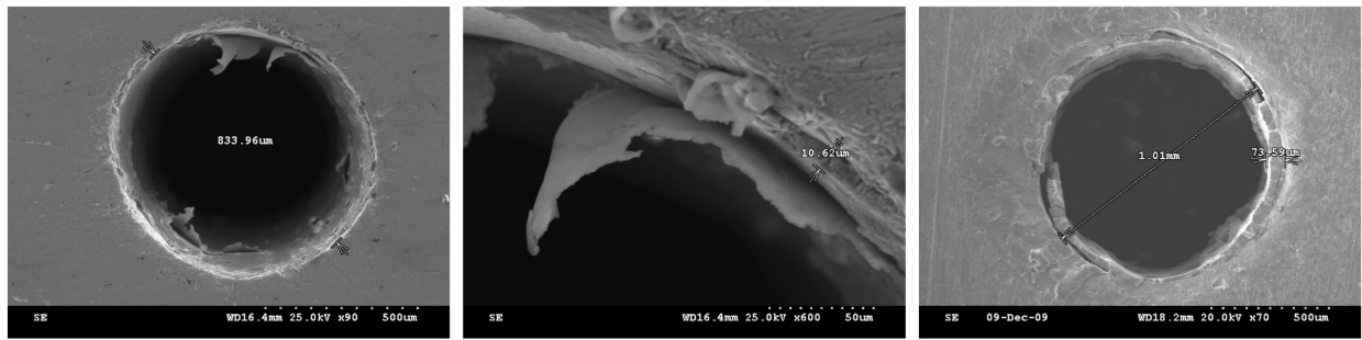
(a)重铸层厚度约 10 \mu\text{m} (优化) (b)薄皮状结构(优化) (c)重铸层厚度约 73 \mu\text{m} (未优化)
