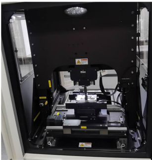
图 10 定子线棒研磨整体平台 Fig. 10 Overall platform for stator bar abrasiveness
