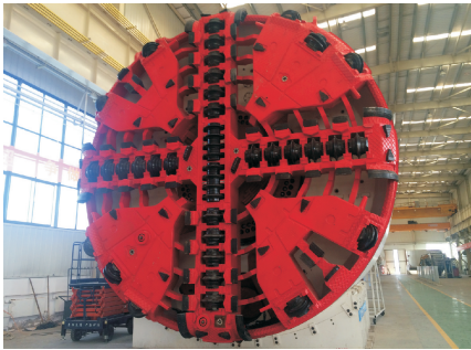
图 11 某型土压平衡盾构机刀盘面板结构 [5] Fig. 11 The cutterhead panel of a certain earth pressure balance shield machine [5]
