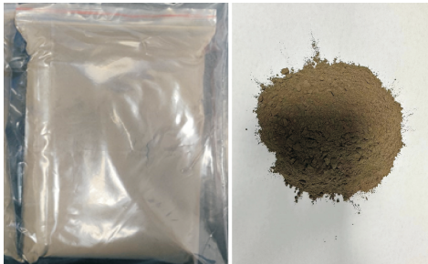
图 2 河北某钢厂产生的锌灰 Fig. 2 Zinc ash produced by a steel factory in Hebei
