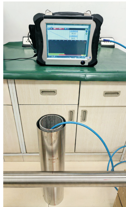
图5 压力管-排管-LISS 管间距脉冲涡流检测实验装置 Fig. 5 Experimental setup of pulse eddy current testing for pressure tube-calandria tube-LISS tube spacing
