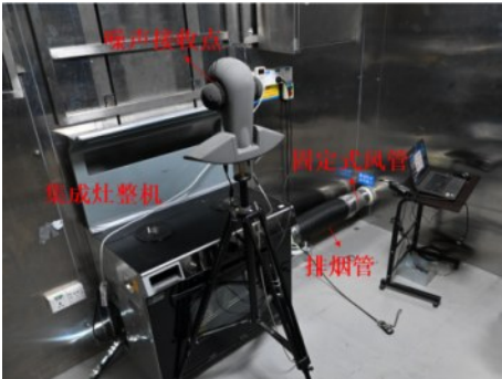
图 8 集成灶工作噪声测试台 Fig.8 Testing platform of aerodynamic noise of integrated stove at the working condition
