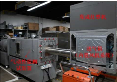
图 7 集成灶气动性能测试台 Fig.7 Testing platform of aerodynamic performance of integrated stove
