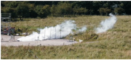
图 5 液氢泄漏实验云团 Fig. 5 An experimental cloud of liquid hydrogen leakage
