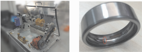
(a)实验台 (b)外圈预制微弱故障
